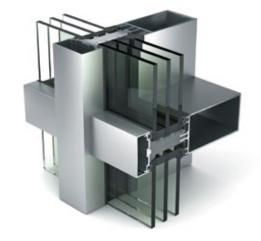
A passive house does not require an active heating system and therefore relies heavily on the thermal insulation and air-tightness of the façade. Based on the standard series, WICTEC 50 is certified for aluminium/glass façades suitable for passive houses at minimal additional cost. The thermal insulation is improved to passive-house quality with a  $\rm U_f$  value of 0.74 W/(m²K) when using triple glazing and an easy-to-install thermal break profile.
